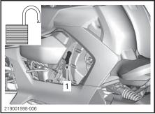
1. PARK lever in unlock position (disengaged)
