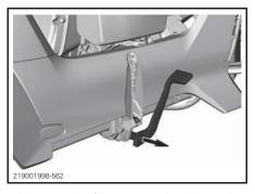
Lower the footpeg and validate that the driver is able to apply the full stroke of the brake pedal.
