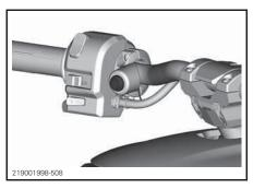
The hazard warning flashers may be activated any time even if the engine is not running. The flashers will drain the battery if they are use for an extended time.
