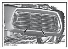
3. Roll up the end of the front fascia extensions to release the rear retaining tabs.
