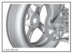
Install the conical washer and the center lock wheel nut
