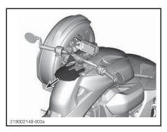
4. Unscrew slowly the fuel reservoir cap counterclockwise to remove it.
