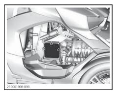
1. Remove the screw retaining the bottom of the CVT air filter housing.
