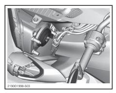
4. Turn the bulb stopper counterclockwise to unlock it.
