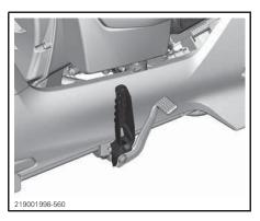
Slide the footpeg and the brake pedal forward or rearward to the desired position.
