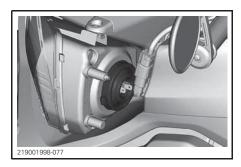
4. Turn the bulb stopper counterclockwise to unlock it.
