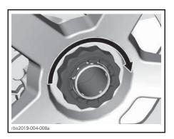
Remove locking device from the wheel hub.
