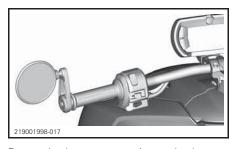
Press the button to activate the horn.
