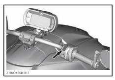
To start the engine, toggle the engine stop switch on the RUN position.
