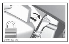
To unlock the park position lever, turn key counterclockwise.
