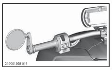
This switch is used to select either the headlights low or high beams
