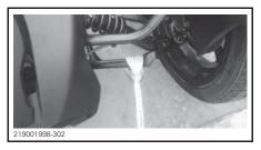
3. Attach the straps to the winch cable.
