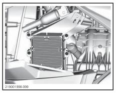
4. Remove the air filter from its housing.
