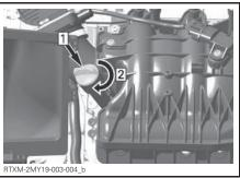
Step 1: Insert dipstick Step 2: Tighten dipstick.
