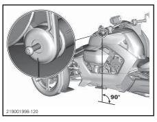
5. Hold the support and tighten the screw.
