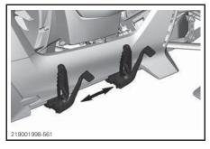
3. Pull the brake pedal and position it in a functional position.
