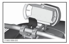
Move the handlebar back and forth until a comfortable position is obtained.
