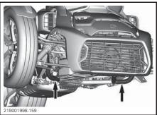
USE THESE TUBES TO LIFT OR SUPPORT THE FRONT OF THE VEHICLE
